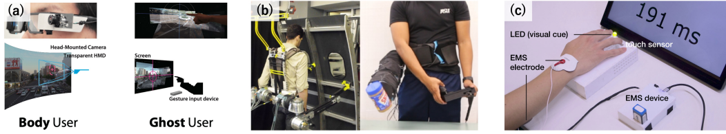
Figure 2.1: Examples of Augmented HCI. (a) JackIn: a vision augmentation system based on a third-person perspective [32]. (b) A wearable robotic limb that enhances human capabilities [33]. (c) Electrical muscle stimulation training that improves reaction time [34].
