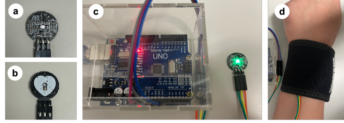
Figure 7.2: The device used to obtain the real-time heart rate. (a) Front of PulseSensor. (b) Back of PulseSensor. (c) Connection between the Arduino and the PulseSensor. (d) Attaching the sensor on the player's wrist.
