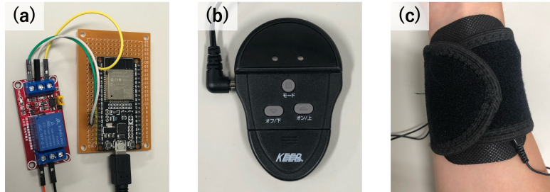
Figure 5.3: EMS device: (a) ESP32 and PETTOYA 554. (b) MEF-38 for power supply. (c) Electrode configuration.
